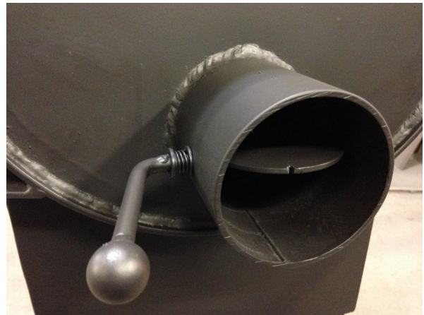
Fig. 2 — Exhaust-gas outlet regulator: OPEN • intensive mode
