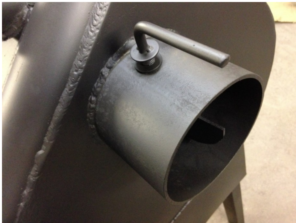
Fig. 1 — Air-supply regulator: OPEN • intensive mode
