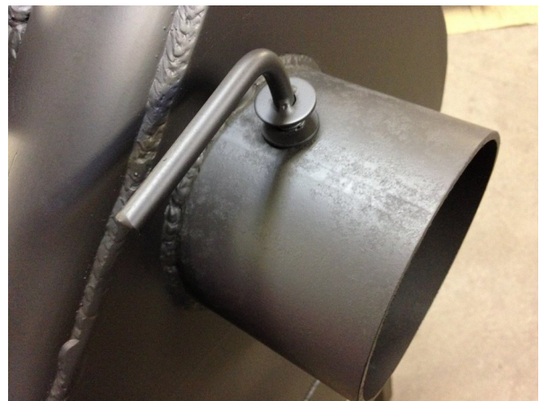
Fig. 4 — Exhaust-gas outlet regulator: CLOSED • gasification mode
