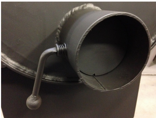
Fig. 3 — Air-supply regulator: CLOSED • gasification mode
